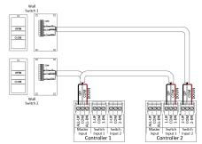
Motor 2 on Controller 2 operate from Wall Switch 1
