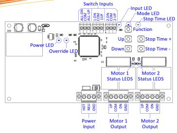
IMPORTANT: If both left and right hand motor configurations are used, UP and DOWN wires for individual motor outputs may need to be swapped in order to function correctly with grouped switches. To verify wiring, all motors should run in the same direction when operated from the onboard UP/DOWN buttons.
